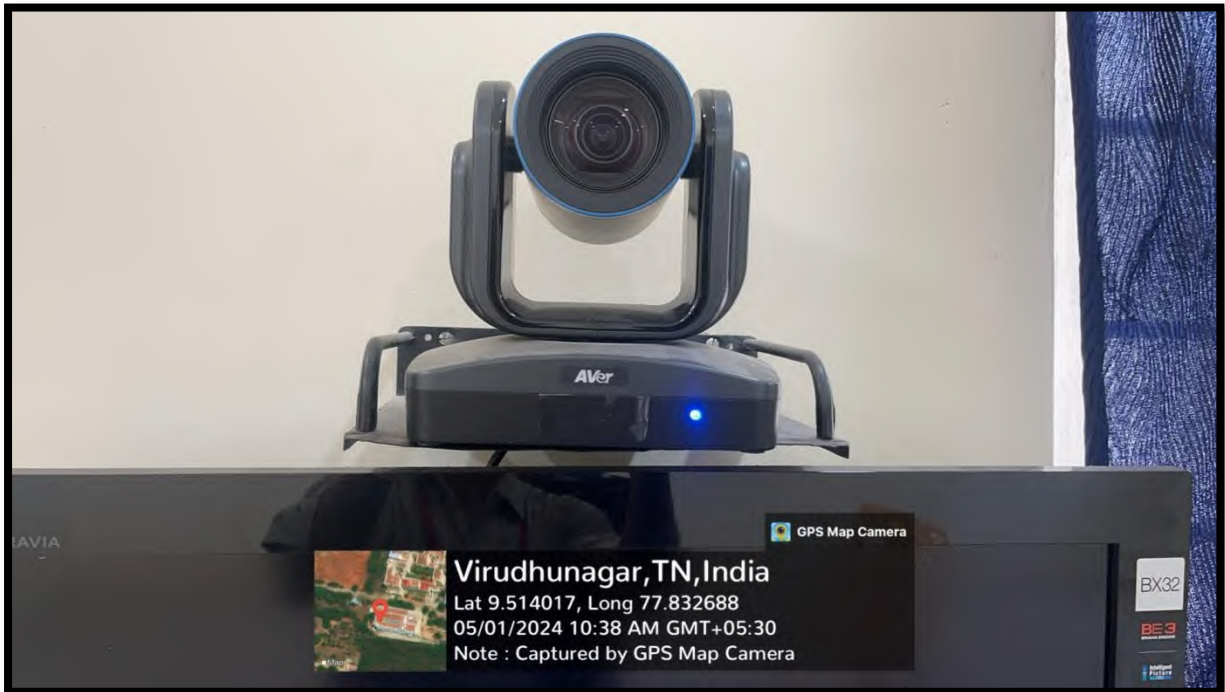
e Cam PTZ IV camera with 12x optical zoom and 4K resolution
